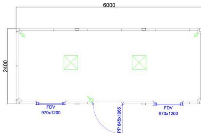
**Dimensions : L = 2400 mm x l = 5980 mm x H 2640 mm - HSP 2350 mm**
